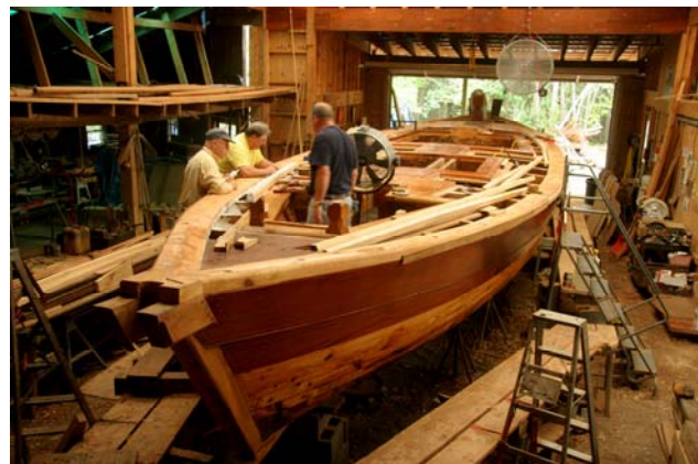
Installing bugeye deck boards with Sidney Dickson, and Tom Huddleston
