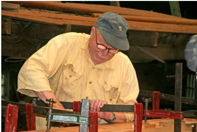
John tightens a deck board clamp
